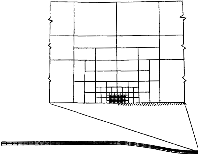
FIGURE 2 Typical deformed mesh of the finite element model for an aluminum specimen.
